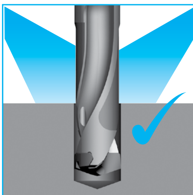
2) In case of external coolant Cutting depth must be 3 \times D or less.
