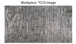
Tearing on Workpiece (Surface Finish Enlarged)
