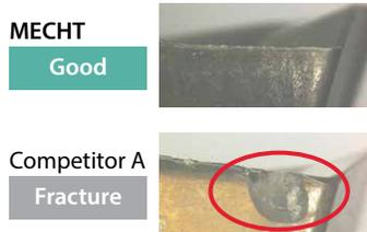
Cutting Conditions : Vc = 130 sfm, D.O.C. x ae = 1.692" x 0.787", fz = 0.0047 ipt, ø50mm (5 Flutes), Wet (External and internal coolant) Workpiece : Ti-6Al-4V Machine : T50
