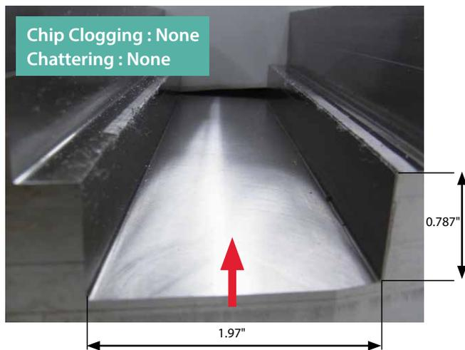
Cutting Conditions : Vc = 130 sfm, D.O.C. x ae = 0.787" x 1.97" (Slotting), fz = 0.003 ipt ø50mm (5 Flutes), Wet (External and internal coolant) Workpiece : Ti-6Al-4V Machine : BT50
