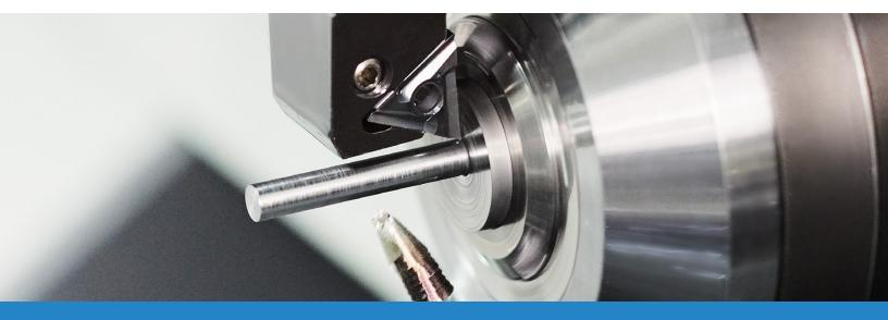
High Precision Machining in a Single Pass with Max Depth of Cut: 0.472" (12mm)
