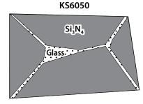
The grain boundary phase contained a high proportion of glass, therefore its toughness will be weakened by cutting heat
