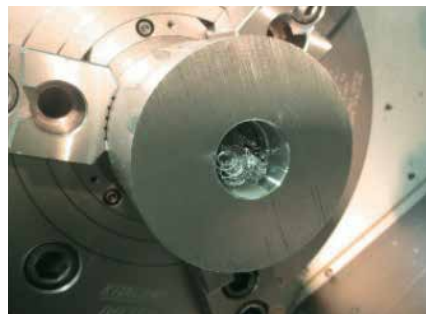
Chip clogging reduces surface finish quality
