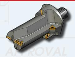
A 34.44mm diameter combination tool on a special threaded shank with facing and chamfer. This tool also utilizes a center insert to break up a thin cast web.
