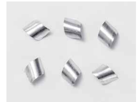
Even Chips with Small Curl Diameter
