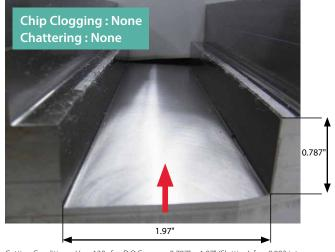
Cutting Conditions : Vc = 130 sfm, D.O.C.  $\times$  ae = 0.787"  $\times$  1.97" (Slotting), fz = 0.003 ipt  $\emptyset$ 50mm (5 Flutes), Wet (External and internal coolant) Workpiece : Ti-6Al-4V Machine : BT50
