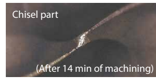
Good without fracture
