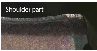
Normal wear condition
